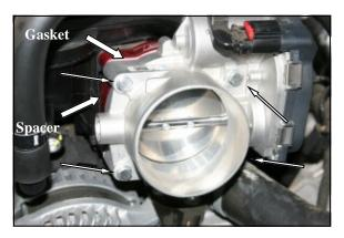
3. Insert the four 6mm x 75mm bolts (#3) with washers (#4) thru the throttlebody, one gasket (#2), and thru the Poweraid Spacer (#1), and into the intake manifold. Tighten all four throttle body bolts evenly, to the manufacturer's specifications. Do Not Over Tighten The Bolts!
